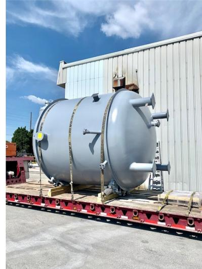
This heavy wall carbon steel pressure vessel went to a refinery in Ohio. The team met an expedited schedule to deliver this vessel before a plant shut down.
