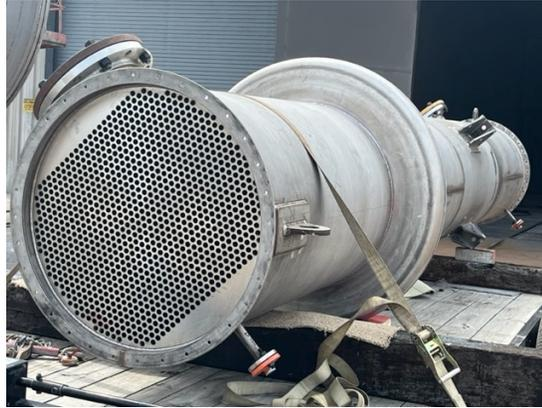
This shell and tube heat exchanger was a TEMA Model- E-34-240 with 2205 duplex tubes that were expanded on the tube to tube sheet joint and also featured an expansion joint on the shell.
