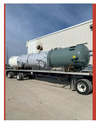
Our team successfully fabricated and shipped this heavy wall pressure vessel that was 72" ID X 30'-0" tangent length with a 2.5" thick intermediate head and full xray, PWHT, mag particle testing, and much more.
