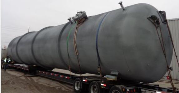
We recently fabricated this pressure vessel that was 10' OD X 50' long and 1" thick made of 516-70 carbon steel and weighing 90,000 pounds for a petrochemical plant in the northeast. This vessel also had a ladder and platform, (3) vacuum rings, and was full x-ray. Nice project!
