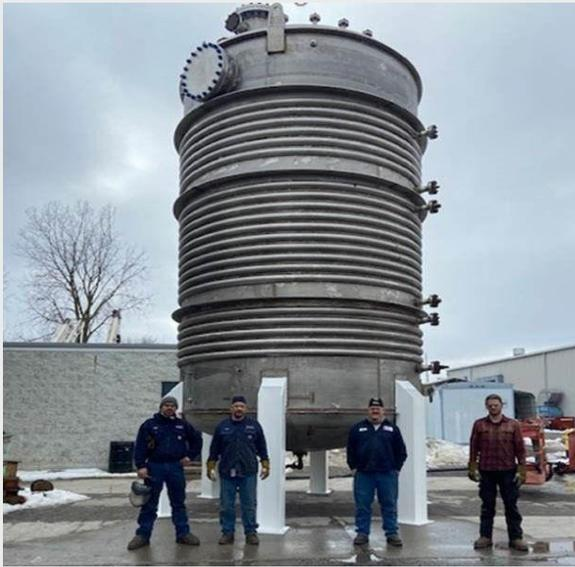
This week we successfully hydro tested this stainless vessel which was 144" ID X 18'-3" tangent length with (4) internal baffles, (3) zones of the half-pipe, and (26) unique nozzles.
