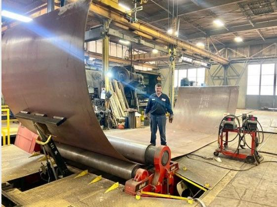
Kennedy Tank veteran **Gary Martin** is rolling a 1/2" thick, 118" wide X 450" long plate for a 50,000-gallon tank we are getting started on in our manufacturing facility.
