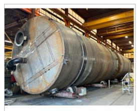
We are mid-fabrication on (2) 14'-6" diameter X 34' long carbon steel water filtration tanks fitted with several internal and external stiffeners.
