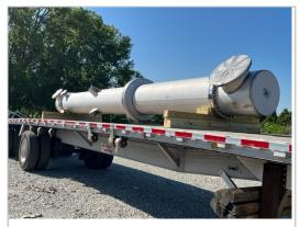
We also built this BEM 23-240 shell and tube heat exchanger that was comprised of 2205 duplex material for both the tubes and tube sheets.
