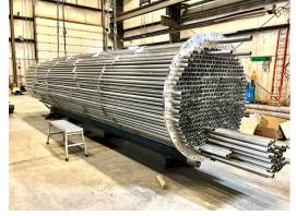
This shell and tube heat exchanger bundle weighed over 20,000 pounds and was put together in our segregated stainless steel building.
