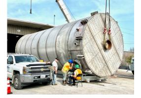
We continue to see more requirements for third-party passivation which is being performed above on a 40,000-gallon stainless steel API 650 shopbuilt tank.
