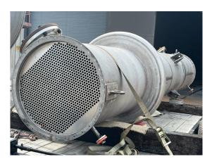
This shell and tube heat exchanger was a TEMA Model- E-34-240 with 2205 duplex tubes that were expanded on the tube to tube sheet joint and also featured an expansion joint on the shell.
