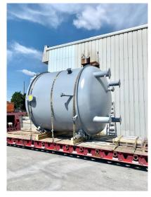
This heavy wall carbon steel pressure vessel went to a refinery in Ohio. The team met an expedited schedule to deliver this vessel before a plant shut down.
