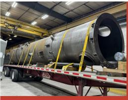
One of the mottos we live by here at Kennedy Tank is **Our Quality is our Customer's Safety** and that was evident on this heavy wall pressure vessel with a 2.5" thick inner head where all 200+ x-rays were passed before post weld heat treatment.
