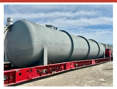
This week we shipped this heavy-wall carbon steel pressure vessel that is 12' -0" I.D. X 56' -0" tangent to tangent length, 2:1 elliptical heads on support saddles and weighing 80,000 pounds.
