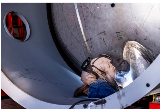
Teammate Anthony Wallace tig welding a bottom nozzle on a stainless steel vessel with a carbon steel skirt.
